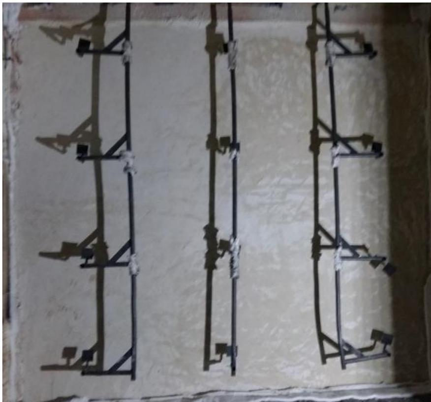
ANNEXE 33 : PHOTO DE LA FACE NON EXPOSEE AU FEU DU MUR AVANT ESSAI
